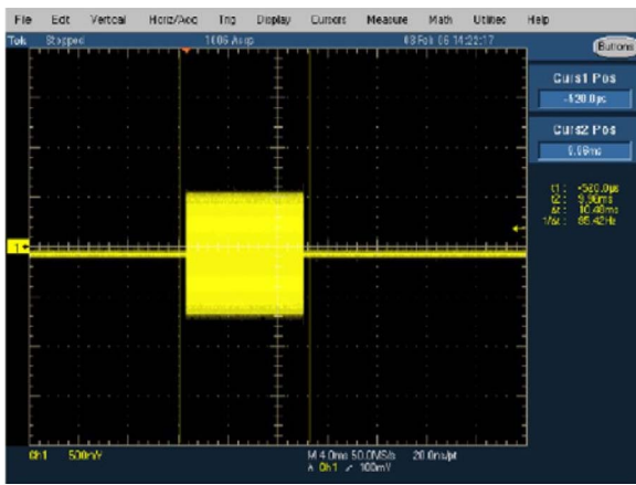
Fig. 9. CE-OFDM signal output with no PAPR [57].
