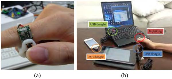
Fig. 7: (a) Prototype of MobiRing (b) System Prototype.
