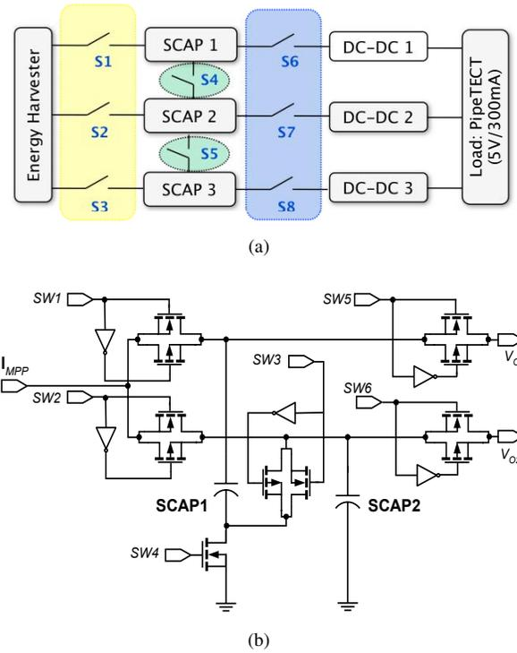
Fig. 3. Dynamic reconfigurable switch array (DRSA): (a) block diagram for three supercapacitors, (b) schematic for two supercapacitors
