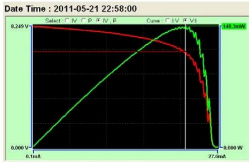
Fig. 5. Measured Solar panel I-V curve.
