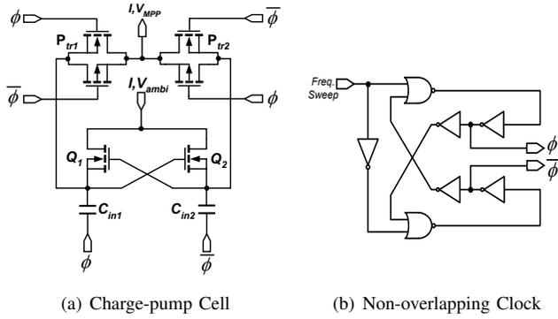
Fig. 2. Charge Pump Configuration
