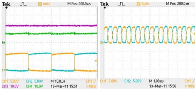
(a) Measured boost-up (b) Non-overlapping clocks @1MHz
