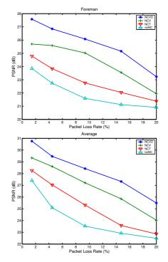
Fig. 5. Video quality observed over wireless channel *Model I*. Average PSNR for *Foreman*, and avg PSNR averaged across all 3 sequences.
