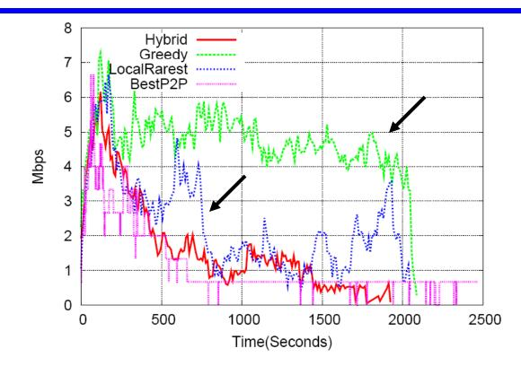
Proposed adaptive hybrid best compromise between low seeder load and jump delay
